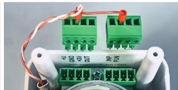
Photo 24. Connecting a wired switch
