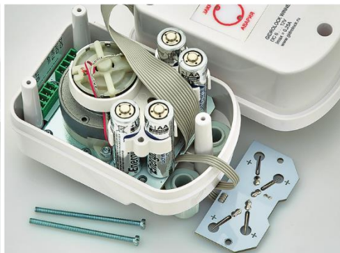
Photo 17. Contact plate is removed, batteries can be replaced
