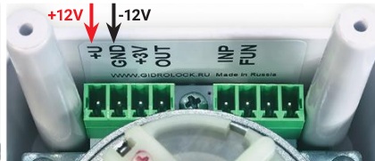
Photo 20. Electric actuator connector terminals for connecting an external +12V power supply unit, a wire switch, combining several electric ball valve actuators into a system
