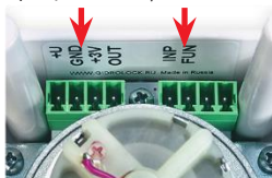
Photo 13. Terminals for connecting wired sensors — INP, GND
