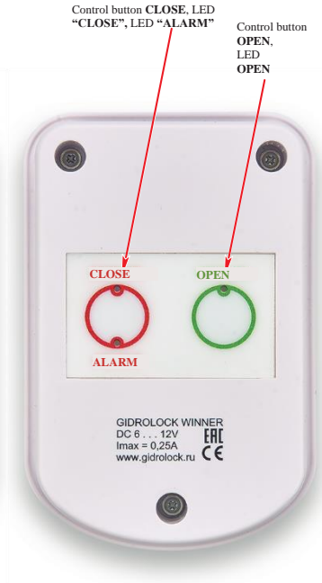
Photo 8. Controls on the electric ball valve actuator body
