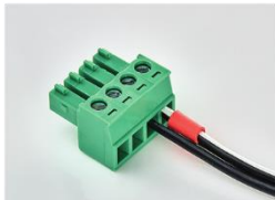
Photo 19. Connecting an external +12V power supply unit to the mating connector of the electric actuator
